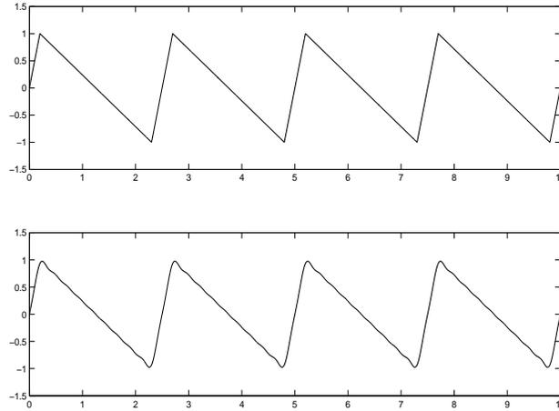
FIGURE 2.7: A vibration and its Fourier approximation,  $m = 6$
