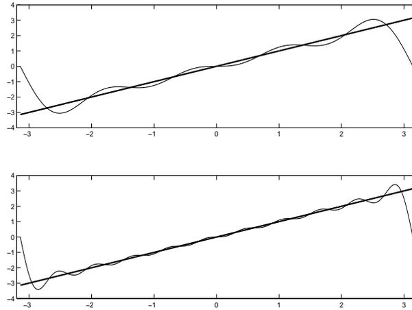
FIGURE 2.5: Fourier approximation of  $g(\theta) = \theta$ ,  $m = 4$  and  $m = 10$
