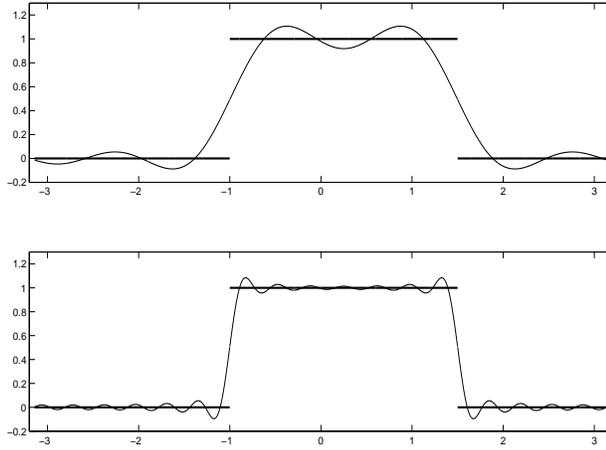
FIGURE 2.4: Fourier approximation of the function (2.73),  $m = 4$  and  $m = 18$
