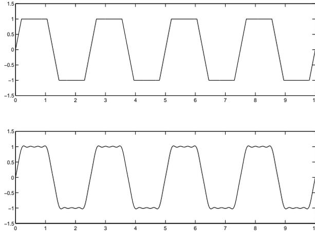
FIGURE 2.6: A vibration and its Fourier approximation,  $m = 10$
